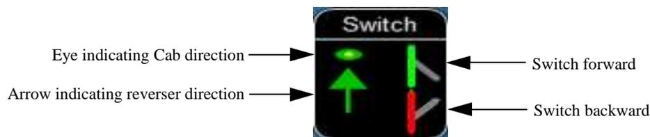
Switch shown in green can be operated, switch shown in red is locked.
