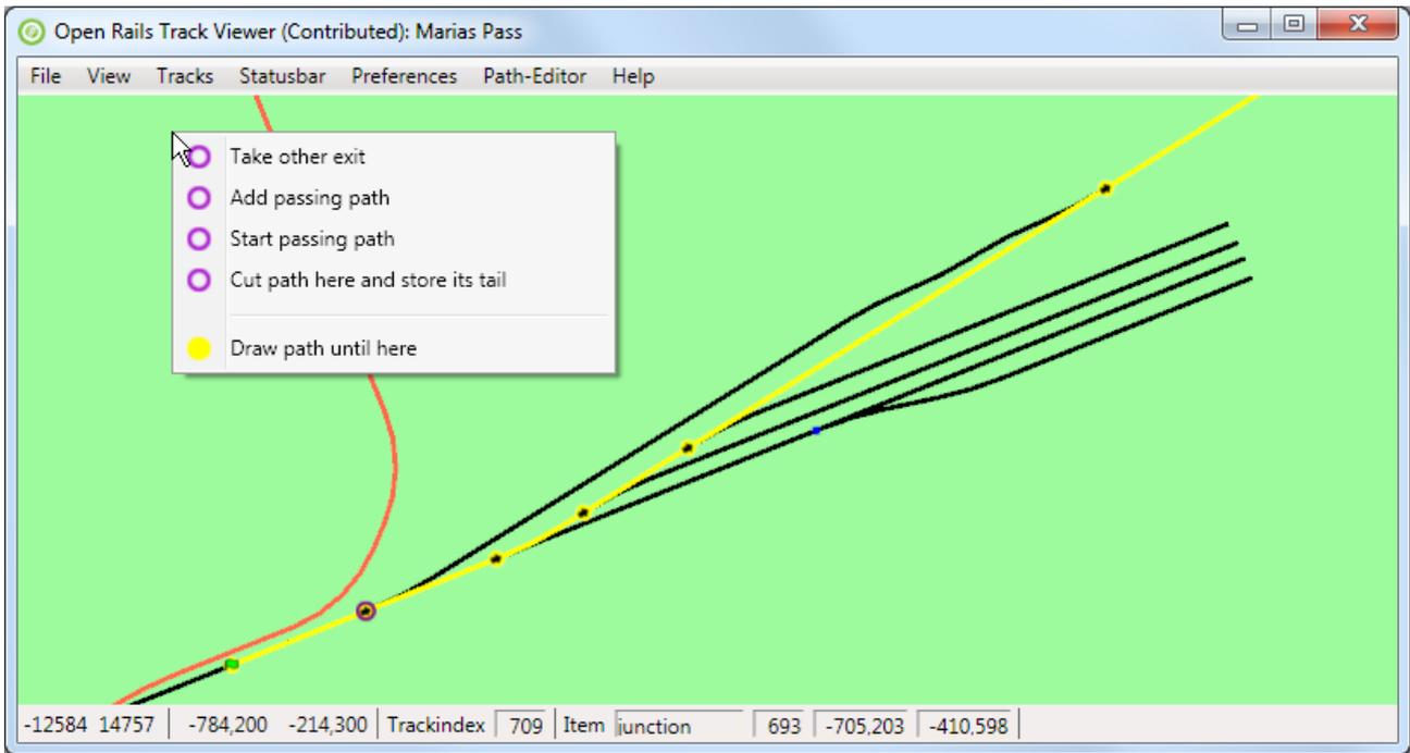
The result is shown below: the passing path has been added (in orange). In this case it is a very simple passing path without any nodes.
