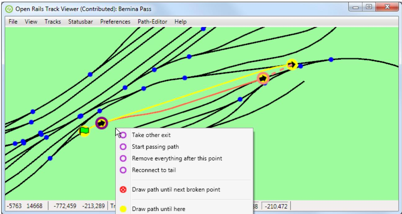
Now that the direction is reversed, it is possible to reconnect to the tail. There is no need to first 'Take other exit'. Just press 'Reconnect to tail'. The result is a fine and completely connected path again:
