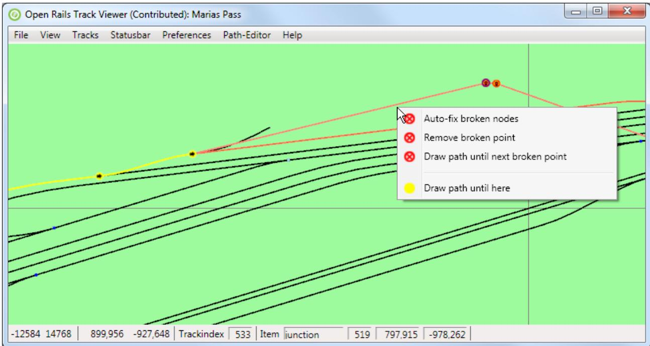
As one can see the path is fine and drawn in yellow until a certain node. Then, on the top right there are two broken nodes. Apparently the tracks have been changed quite a bit after this path was created. Right clicking on one of the relevant nodes (that would be either the broken nodes themselves or the good nodes just before or after the broken path) will have, in the popup-menu, the item 'Auto-fix broken nodes'. Selecting this will auto-fix the broken nodes. The result is then:
