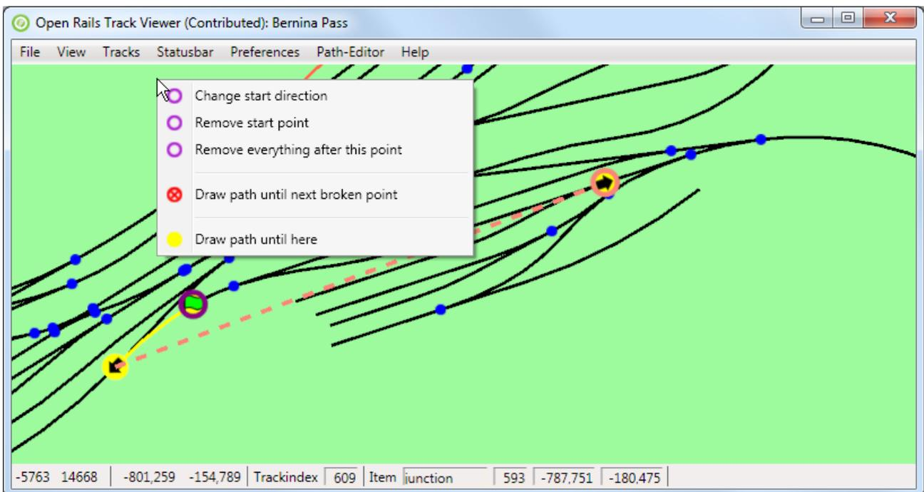
The direction of the start point is to the lower-left. This makes it impossible to auto-fix the path. The obvious solution is to 'Change start direction':
