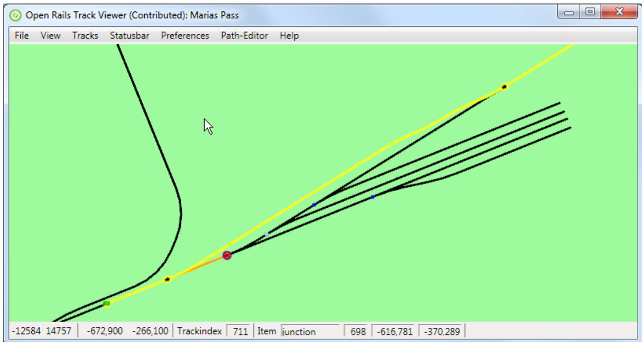
This will create only the first part of a passing path. The path is now broken (as can be seen from a cross through the just created node on the passing path).
