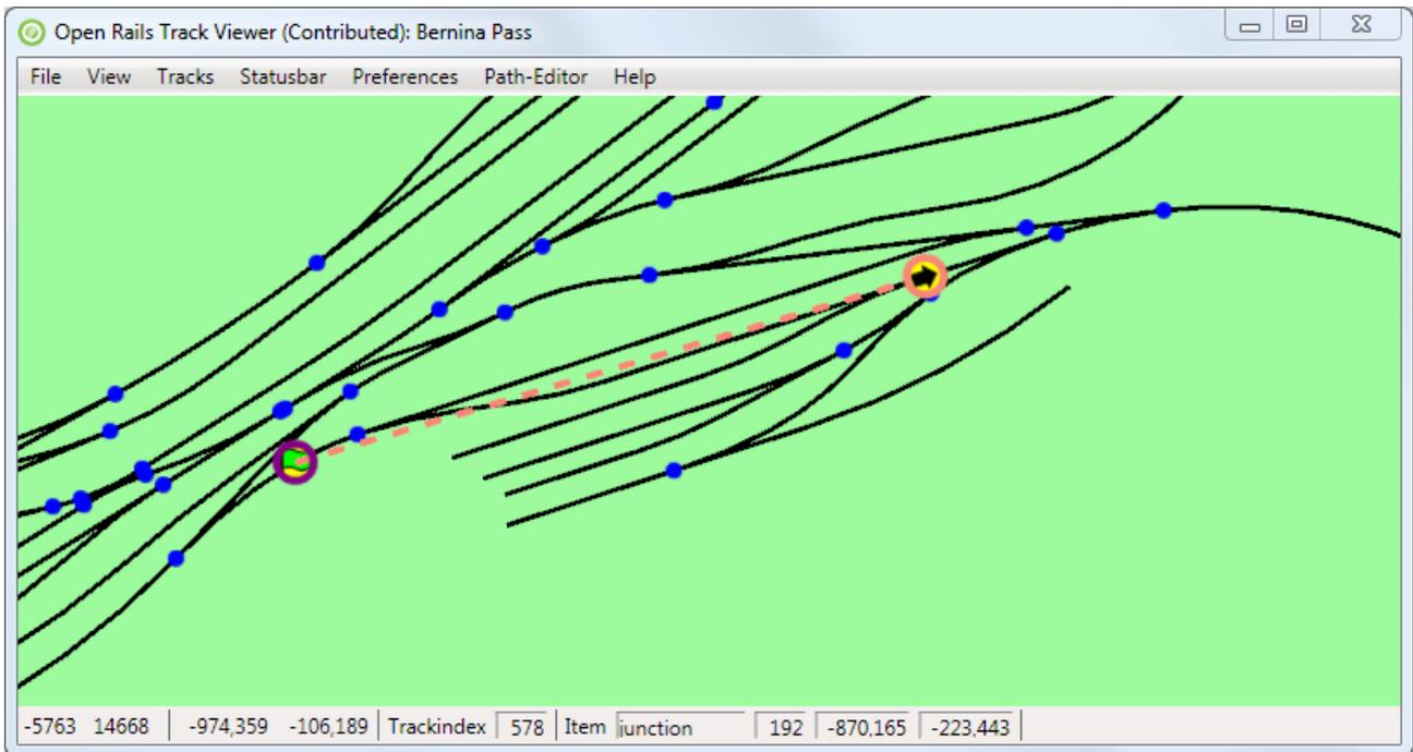
The tail is now drawn using only its first node. Furthermore, there is a dashed line from the last drawn node of the path to the tail. In this way you see where you need to connect again.
