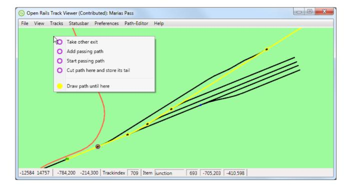
The result is shown below: the passing path has been added (in orange). In this case it is a very simple passing path without any nodes.
