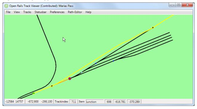
This will create only the first part of a passing path. The path is now broken (as can be seen from a cross through the just created node on the passing path.
