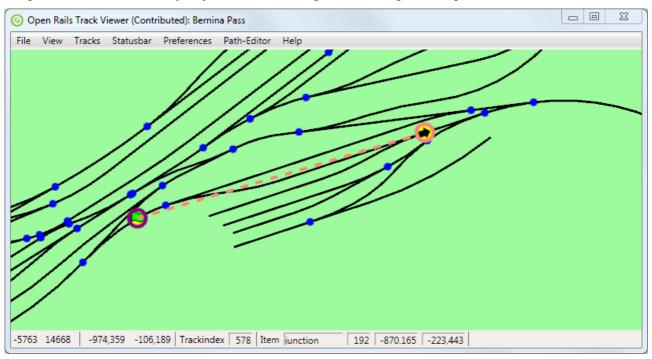
The tail is now drawn using only its first node. Furthermore, there is a dashed line from the last drawn node of the path to the tail. In this way you see where you need to connect again.
