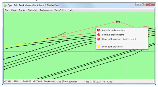
As one can see the path is fine and drawn in yellow until a certain node. Then, on the top right there are two broken nodes. Apparently the tracks have been changed quite a bit after this path was created. Right clicking on one of the relevant nodes (that would be either the broken nodes themselves or the good nodes just before or after the broken path) will have, in the popup-menu, the item 'Auto-fix broken nodes'. Selecting this will auto-fix the broken nodes. The result is then:
