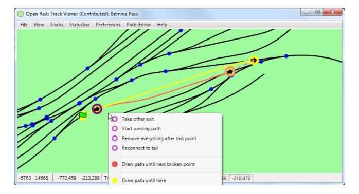
Now that the direction is reversed, it possible to reconnect to the tail. There is no need to first 'Take other exit'. Just press 'Reconnect to tail'. The result is a fine and completely connected path again:
