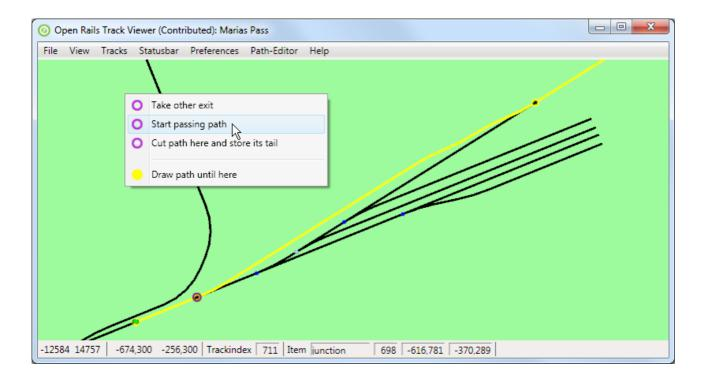
Starting the passing path at the same point, and following only main tracks at each junction would not lead to a reconnect-point, but only to one of the sidings. To create a passing path here the first step is to 'Start passing path':
