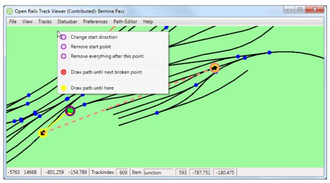
The direction of the start point is to the lower-left. This makes it impossible to auto-fix the path. The obvious solution is to 'Change start direction':
